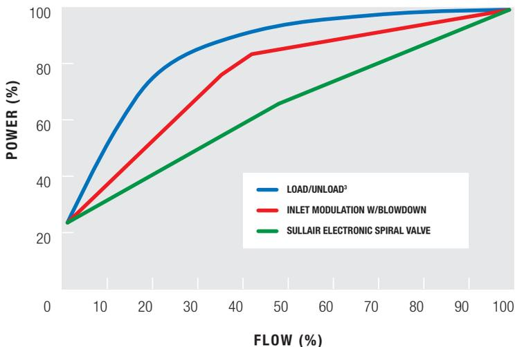
*The costs to operate an air compressor—especially energy costs—can quickly exceed the initial purchase price. Effectively matching compressor production capacity to your facility needs is the best way to save both energy and money.*
