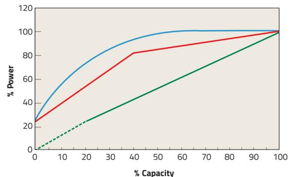
— Single-Stage Lubricated Load/Unload (based on one gallon/storage per cfm)
